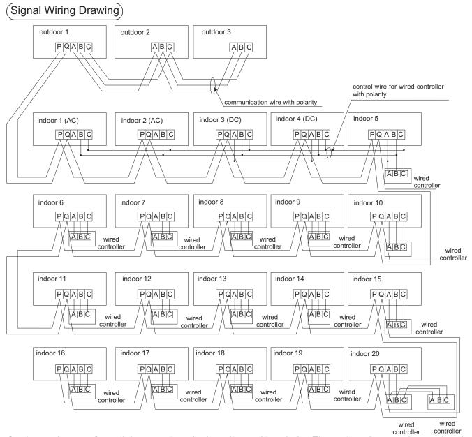
Outdoor units are of parallel connection via three lines with polarity. The main unit, central control and all indoor units are of parallel connection via two lines without polarity.
