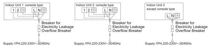
Indoor units and outdoor units should be connected to the power source separately. Indoor units
