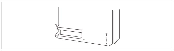
• Once refrigerant piping and drain piping connections are complete, fill the gap of the through hole with putty. Attach the front panel and front grille in their orginal positions once all connections are complete.
