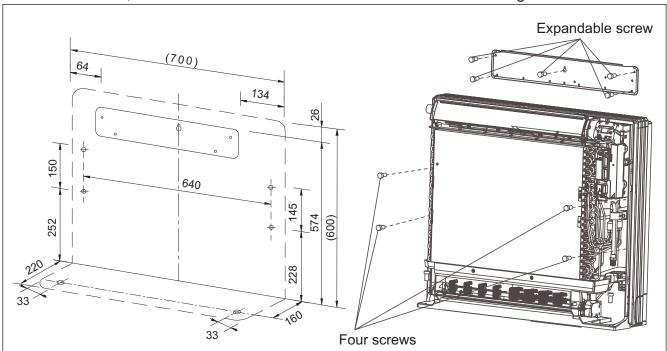
Remove the front panel, then use two fastening screws to fix the unit on the floor. As the figure shown.
