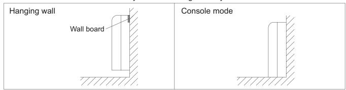
• Fix the wall board, then use four screws to fix the unit on the wall. As the figure shown.
